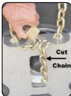
**2:** As per the picture on the right place one side of the padlock's Shackle through the last link on the left. Holding the Shackle and Chain on the left use your right hand to pull any slack out of the Chain. Then place the other side of the Shackle through a link on the right side of the Chain to ensure the Steel Shield is as tight as possible to the Wheel.
